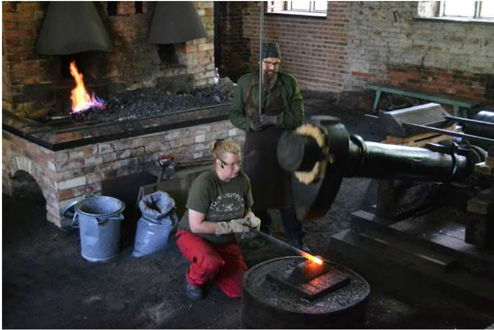
6. Demonstration of the water powered bar hammer at the Upper Forge in Strömfors.
