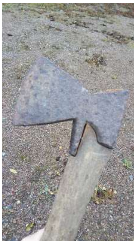
14. A rusty Strömfors model felling axe. The corrosion has completely eaten away the stamp on the left side of the blade.
